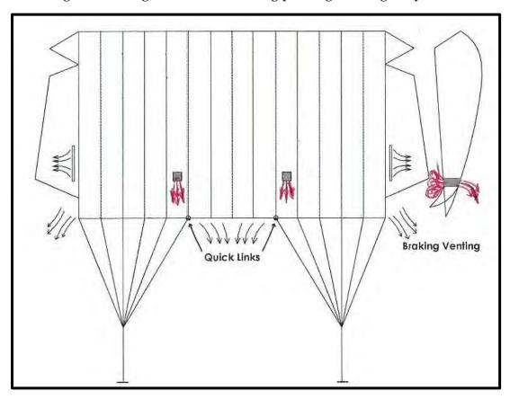
In addition, the inner ( $6^{th}$ ) line is attached with a quick-link, allowing the competitor to move it to the  $5^{th}$  line attach point in a matter of seconds—most particularly if they anticipate highwind jumps. With the  $6^{th}$  line moved to the  $5^{th}$  line attach point, forward speed increases approximately 1 m/s (2.2 mph). Voilà! . . . you have the best of both steering geometries, normally 6-line with the special "Plus Mod" vents; then for high-winds—5-line braking.
